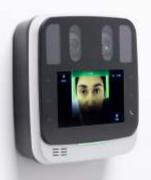
Innovative face positioning feedback provides outstanding subject ease-of-use at capture range of 35 to 45 cm
